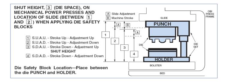
If you know the weight of the press slide and everything attached to it select safety block that matches that number allowing for a safety factor of two. If this number is not known the weight to be supported can be calculated using the formula shown below.
